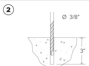
Drill 3/8" diameter holes 3" deep into surface. Make sure the holes are at least 3" away from any cracks in the base material.
