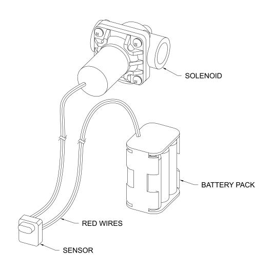
OUTDOOR BOTTLE FILLER PARTS BREAKDOWN DRAWING: NOTE: See page 11 for table of part numbers corresponding to drawing below.
