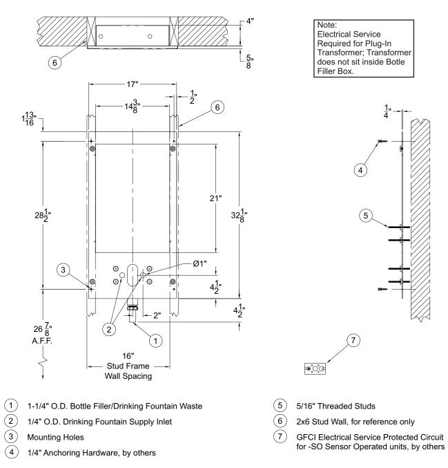
**NOTES:** Dimensions shown for Adult ADA compliant installation. For Child ADA compliant parallel approach installation, decrease height of installation by 3 inches. Provide clear floor space as required. Adjust vertical dimensions as required to comply with federal, state, and local codes.
