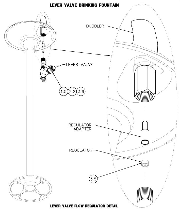
Refer to drawing #9940-205-0M1 for Valve Maintenance Instructions numbered solutions detailed above.
