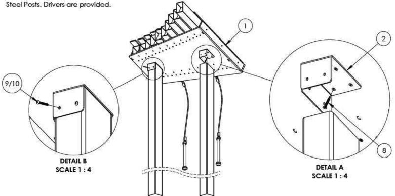
Step 1: Excavate two 10" diameter holes, 36" deep, and 24" on center at the installation location. Contractor can modify Post to desired height. Post Length = Frost Depth (36" Recommended) + Finished Post Height
