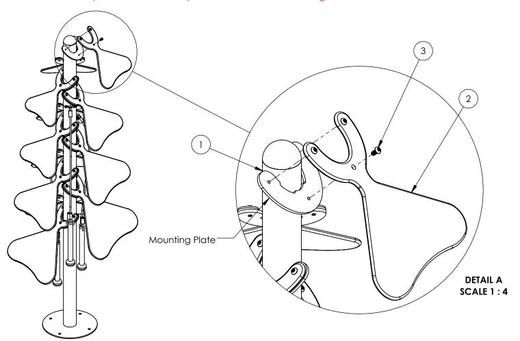
**Step 1:** Determine installation location. Verify concrete footing is a minimum of 24" long x 24" wide x 6" thick. If the concrete pad is at an angle, steel washers are required to act as shims (Shims not provided). If there is not already an existing pad, approximately (3) 80lb. bags will be needed. Allow concrete to cure per concrete manufacturers guidelines. (If a In-Ground appearance is desired recess the concrete pad 4" below finished grade)
