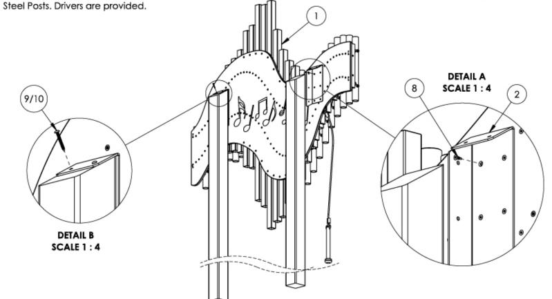
Step 1: Excavate two 10" diameter holes, 36" deep, and 32" on center at the installation location. Contractor can modify Post to desired height. Post Length = Frost Depth (36" Recommended) + Finished Post Height
