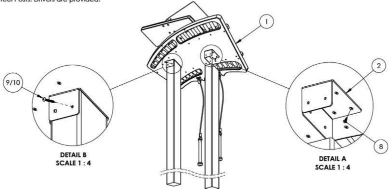
Step 1: Excavate two 10" diameter holes, 36" deep, and 18" on center at the installation location. Contractor can modify Post to desired height. Post Length = Frost Depth (36" Recommended) + Finished Post Height
