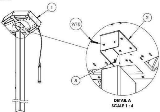
Step 1: Excavate one 10" diameter hole, 36" deep, at the installation location. Contractor can modify Post to desired height.
