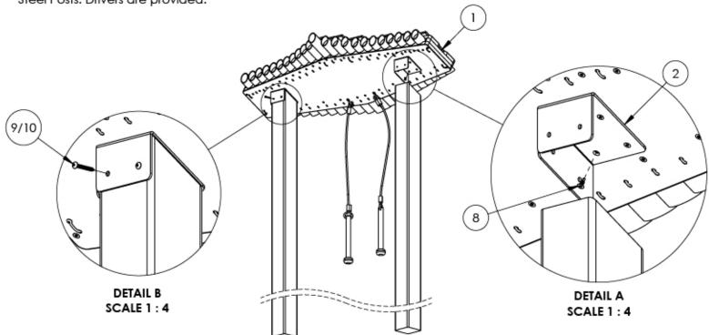
Step 1: Excavate two 10" diameter holes, 36" deep, and 32" on center at the installation location. Contractor can modify Post to desired height. Post Length = Frost Depth (36" Recommended) + Finished Post Height
