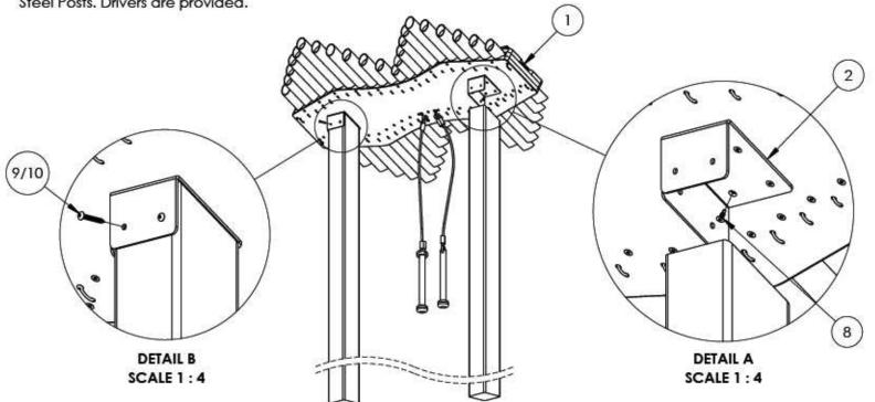
Step 1: Excavate two 10" diameter holes, 36" deep, and 30" on center at the installation location. Contractor can modify Post to desired height. Post Length = Frost Depth (36" Recommended) + Finished Post Height
