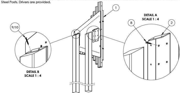
Step 1: Excavate two 10" diameter holes, 36" deep, and 18.625" on center at the installation location. Contractor can modify Post to desired height. Post Length = Frost Depth (36" Recommended) + Finished Post Height
