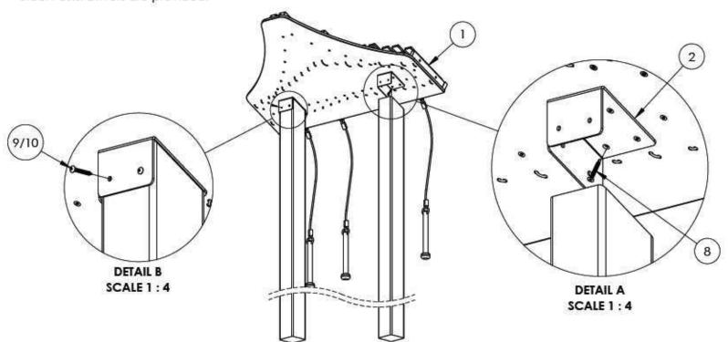
Step 1: Excavate two 10" diameter holes, 36" deep, and 25.5" on center at the installation location. Contractor can modify Post to desired height. Post Length = Frost Depth (36" Recommended) + Finished Post Height
