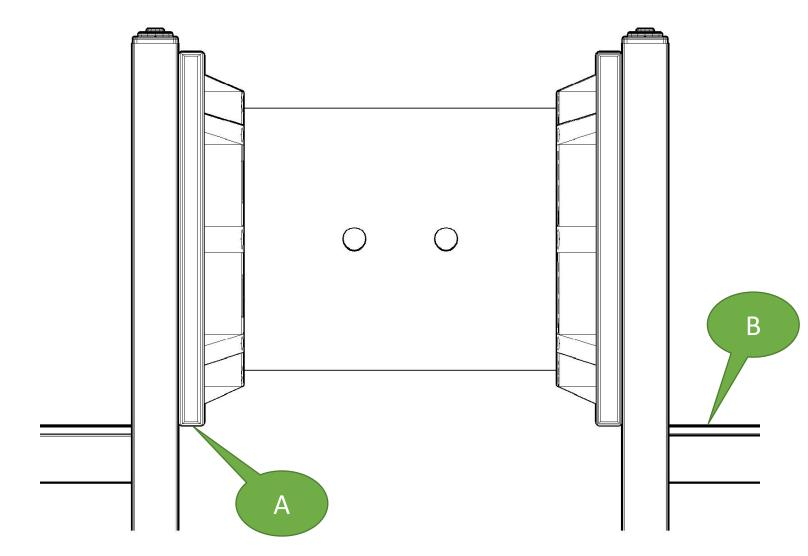
Once the tunnel is lined up properly, pre-drill through the plastic tunnel, at the approximate locations marked below with a 3/16" bit, and into the post. Then fasten a total of (12) 5" RSS SS Screws with washer (3 per side) through the same locations on the crawl tunnel panel and into the 6x6 post.
