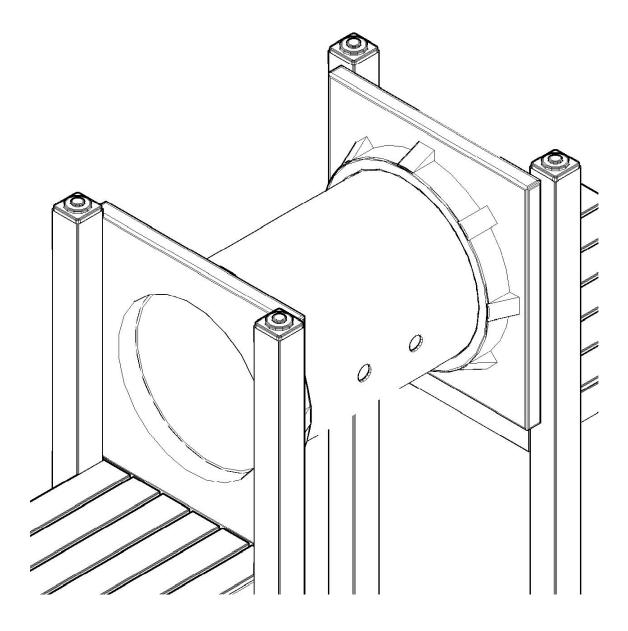
To ensure proper placement of the tunnel before fastening make sure that the flat side of the bottom of the tunnel panel (A) is installed within a 1'' + /- from the top of the deck platform (B).
