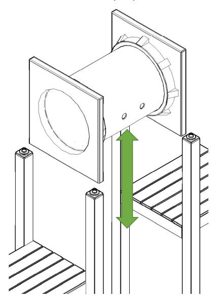
When installing a crawl tunnel please reference the play structure footer drawings for proper footing dimensions associate with the kind of tunnel you are installing. All crawl tunnels whether straight, curved, or inclined, fasten in the exact same manner and this installation can be used as reference for your particular tunnel.
