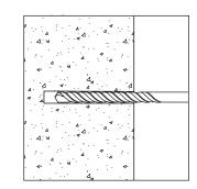
Sleeve anchors: Drill holes 2" deep with 1/2" diameter drill bit. Wedge anchors: Drill holes 3" deep with 3/8" diameter drill bit. Lag screws: Drill holes 3" deep with 9/32" diameter drill bit. Titen anchor: Drill holes 3" deep with 3/8" diameter drill bit. Concrete spikes: Drill holes 3" deep with 3/8" diameter drill bit.
