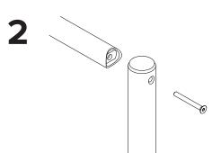
Ensure the countersunk side of the vertical members is facing out and insert the countersunk hex bolts through the vertical member, threading into the brass colored, threaded riv-nut fixed into the horizontal cross bar.
