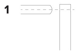
Align the horizontal cross bar and vertical members so the bolt holes line up.
