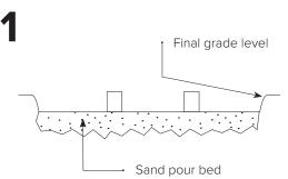
Place corrosion resistant sleeve (min. 4" inside diameter) in sand pour bed in exact location where rack will be installed. Make sure top of sleeve is at same level as desired finished concrete surface. Fill sleeve with sand to keep it in place and prevent it from filling with concrete.
