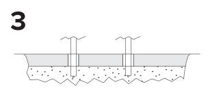
After appropriate cure time, dig out sand from sleeves and insert racks, making sure they are level and at the appropriate height. Pour in Por-Rok or epoxy grout and allow to set.
