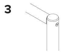
Tighten the countersunk bolts with the appropriate hex key until there the countersunk head seats in the countersunk hole on the vertical member, and so there is no play between the bolted components.
