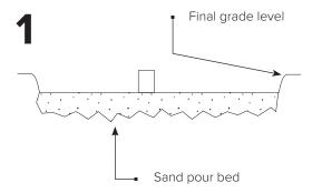
Place corrosion resistant sleeve (min. 3" inside diameter) in sand pour bed in exact location where rack will be installed. Make sure top of sleeve is at same level as desired finished concrete surface. Fill sleeve with sand to keep it in place and prevent it from filling with concrete.
