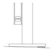
Place rack (and washers to level rack if necessary) over holes.
