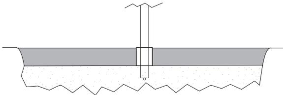
After appropriate cure time, dig out sand from sleeves and insert racks, making sure they are level and at the appropriate height. Pour in Super Por-Rok or epoxy grout and allow to set.
