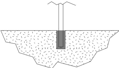
Place rack into holes, making sure the rack is level until the grout has set. 33"-36" of the rack should remain above the surface.
