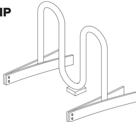
An easy way to brace the rack while the grout sets is to bolt two 1x4" boards together at one end and clamp them onto the rack like a clothes pin.
