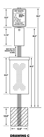
Using a post hole digger, auger, or shovel, prepare a footing hole 12 inches wide and 3a 12 inches deep.
