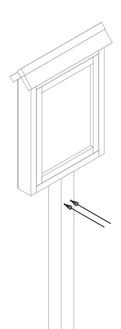
Place the Literature Rack in the desired location on the installed Message Center post and mark the two holes. Remove the Literature Rack and pre-drill the two holes using an 1/8" drill bit going about 3/8" into the 4x4 post.
