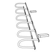
Once nuts are on, tip assembled rack over and use a 9/16" socket to tighten nuts. Before fully tightening nuts, make sure the racks are straight on beams. If using tamper resistant nuts, use access tool to tighten nuts. Do not overtighten the tamper resistant nuts. Tip rack upright.
