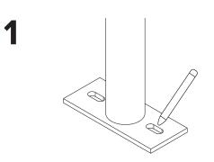
Place the rack in the desired location. Use a marker or pencil to outline the holes of the flange onto the base material.
