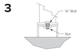
Put bolts through Hoop Rack flange holes and beams so bolt head faces up. HAND tighten the nuts using new flange nuts.
