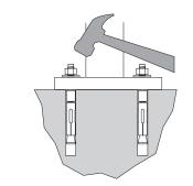
Thread nuts onto anchors, leaving approximately 1/4" of the anchor protruding, and tap into surface. Tighten nuts down to secure rack.
