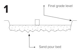
Place corrosion resistant sleeve (min. 3" inside diameter) in sand pour bed in exact location where rack will be installed. Make sure top of sleeve is at same level as desired finished concrete surface. Fill sleeve with sand to keep it in place and prevent it from filling with concrete.
