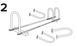
Place Hoop Racks on beams so holes in rack flanges line up with beam slots
