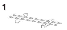
Lay out the two channel beams where the rack will be placed. Place the two beams on top of the two blocks of wood so that the open part of the channel faces the ground.
