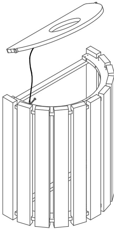
Step 4: If you would like to take advantage of the supplied Lid Lanyard, just remove the desired screw from the top rail and re-secure it with the lanyard attached. Just remove the screw in the lid if you would like to forgo the use of the Lid Lanyard.
