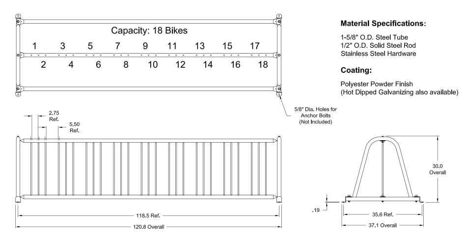
BIKE RACK ASSEMBLY, GRID TYPE, 18 BIKE, 10 FT MODEL: BRG18-P (Painted Frame)
