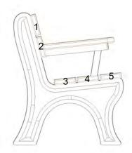
Fig #1: In order to make the assembly of this Economizer Traditional Bench easier while going through the assembly process the board positions are numbered
