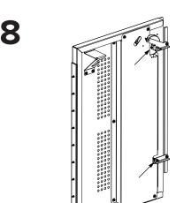
The gap between the door and latch bar may need to be adjusted to properly engage the door frame. This can be done via the ½" bolt that tightens against the handle spindle and the 5/16" nuts at the other pivot point.
