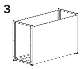
Place the floor panel in the locker and attach to the side panels with (6) 5/16" x .75" carriage bolts, washers, and locknuts. Attach to the door frames with (6) 5/16" x 2.25" carriage bolts, washers, and locknuts. Add the remaining (4) 5/16" x 2.25" carriage bolts, washers, and locknuts that attach the side panels to the door frames. Leave all locknuts finger-tight.
