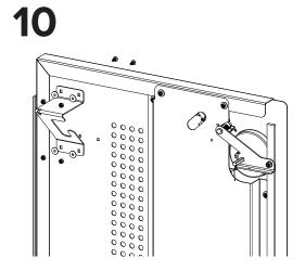
If a gear hook is needed, attach the gear hook to the door back with (4)  $\#10 \times .50$ " carriage bolts, washers, and locknuts.
