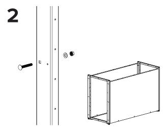
Attach (2) side panels to the (2) door frames with (12) 5/16" x 2.25" carriage bolts, washers, and locknuts. Omit the (4) bottom bolts for now. Leave locknuts finger-tight
