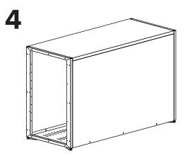
Place the roof panel on the locker and attach to the side panels with (6) 5/16" x .75" carriage bolts, washers, and locknuts. Attach to the door frames with (6) 5/16" x 2.25" carriage bolts, washers, and locknuts.
