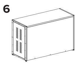
Attach the back panel to the rear door frame with (10)  $\#12 \times 34$ " self-drilling screws. Pilot holes are present but may be partially filled with zinc. Screwing is done from inside the locker.
