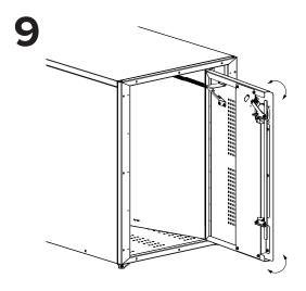
If any twist needs to be taken out of the door, loosen the #10 locknuts, set the door, and retighten.
