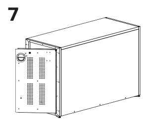
Attach the door assembly with (8) #12  $\times$  34" self-drilling screws. Pilot holes are present but may be partially filled with zinc.
