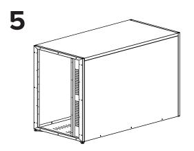
Place the roof panel on the locker and attach to the side panels with (6) 5/16" x .75" carriage bolts, washers, and locknuts. Attach to the door frames with (6) 5/16" x 2.25" carriage bolts, washers, and locknuts.
