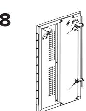
The gap between the door and latch bar may need to be adjusted to properly engage the door frame. This can be done via the ¼" bolt that tightens against the handle spindle and the 5/16" nuts at the other pivot point.
