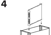
Place the divider panel in the locker and attach to the door frames with (20) #12  $\times$  34" self-drilling screws and 14" washers. Pilot holes are present but may be partially filled with zinc.
