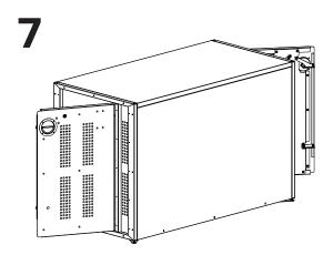
Attach each door assembliy with (8) #12 x  $^{3}4$ " self-drilling screws. Pilot holes are present but may
