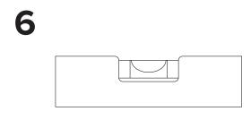
Check that the locker is level and square. Tighten all hardware.
