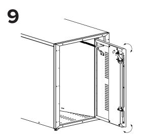
If any twist needs to be taken out of the door, loosen the #10 locknuts, set the door, and retighten.
