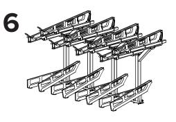
Place the bottom Lower and Upper Trays in position and secure at the rear with (1)  $3/8" \times 1"$  carriage bolt, 3/8" washer, and 3/8" nut each. Secure at the front with (1)  $3/8" \times 3"$  wedge anchor each.
