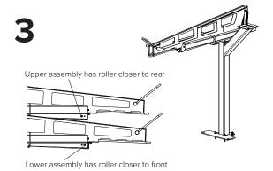
Place the lower Cantilever Assembly on the lower Upright position and secure with (4)  $\frac{1}{2}$ " x 1.25" carriage bolts,  $\frac{1}{2}$ " washers, and  $\frac{1}{2}$ " nylock nuts.
