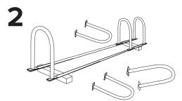
Place Hoop Racks on beams so holes in rack flanges line up with beam slots.
