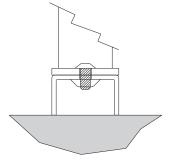
Put bolts through Hoop Rack flange holes and beams so bolt head faces up. HAND tighten the nuts using new flange nuts.
