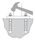
Thread nuts onto anchors, leaving approximately 1/4" of the anchor protruding, and tap into surface. Tighten nuts down to secure rack.
