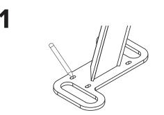
Place the rack in the desired location. Use a marker or pencil to outline the holes of the flange onto the base material.
