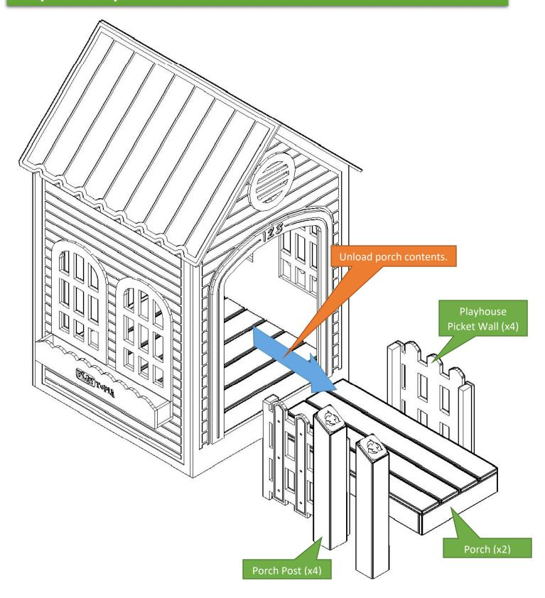
Locate the porch posts and fasten them to the porch as shown below, using (4) 5/16" x 3-1/8" RSS SS Screws.
