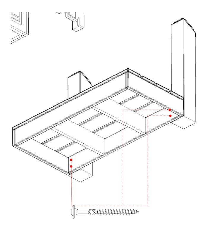
Once posts are fastened, slide porch up against CozyTown Playhouse and fasten together underneath the platforms with (3) 5/16" x 3-1/8" RSS SS Screws.
