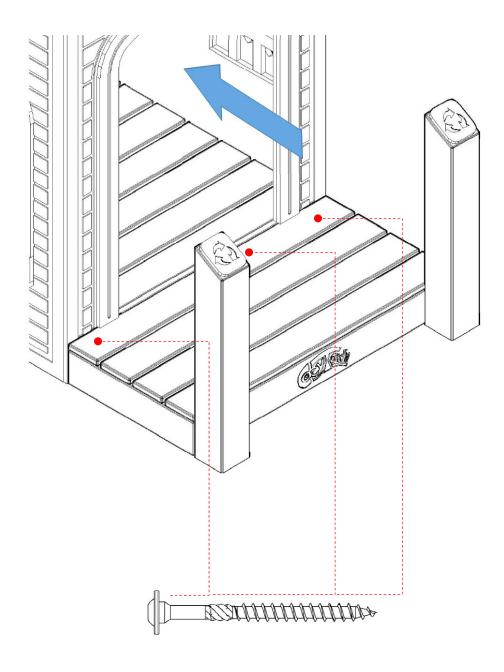
With the porch and posts in place place the picket walls between the playhouse wall and porch post and fasten with (4) 3-1/8" RSS SS screws per picket wall into the wall of the playhouse and into the posts.
