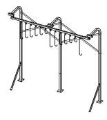
Insert the Track Rack or Bike File assembly into the Channel Supports and secure. See Track Rack or Bike File instructions for more detail.
