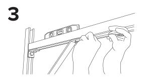
Make sure the horizontal Slotted Track is level. Adjust if necessary.
