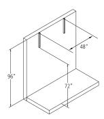
Mount 24" Slotted Tracks vertically to the wall with the appropriate anchors. Use a level for greatest accuracy. The bottom edge of the Slotted Track should be approximately 72" off the floor. The Slotted Tracks should be 4' apart from each other, and the end Slotted Tracks should be 2' from the eventual position of the end of the Trolley track.
