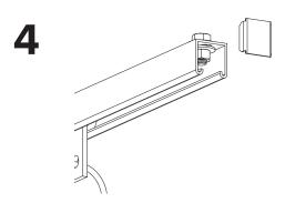
Apply hex head cap screw, washers and nut into last hole at end of the 96" Slotted Track and hammer in End Cap.
