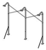
A) For single-sided units, attach Knee Braces to the first Upright and then every other Upright with 3/8" x 3" bolts, 3/8" washers, 3/8" lock washers, and 3/8" nuts. Anchor each Knee Brace by drilling a 3/8" hole and fastening with a wedge anchor.
