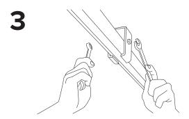
Secure the Channel Trolley Supports onto the 96" Slotted Track by tightening the Hex Head Cap Screws and Flange Nuts through the holes in the Channel Trolley Supports.
