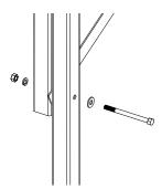
B) For double-sided units, fasten the Double-sided Uprights and Upright Braces to the Uprights with 3/8" x 3" bolts, 3/8" washers, 3/8" lock washers, and 3/8" nuts.
