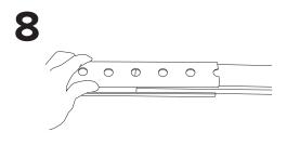
If splicing an additional length of track, slide the Splice Slotted Track over the last 6" of the 96" Slotted Track.
