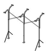
B) For double-sided units, attach (2) Knee Braces to the first Upright and then every other Upright with 3/8" x 3" bolts, 3/8" washers, 3/8" lock washers, and 3/8" nuts. Anchor each Knee Brace by drilling a 3/8" hole and fastening with a wedge anchor.
