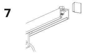
If no more Track Racks are going to be spliced together, apply hex head cap screw, washers, nut and End Cap in the open end of the Slotted Track to keep trolleys from sliding out.
