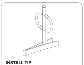
An easy way to brace the rack while the grout sets is to bolt two 1x4" boards together at one end and clamp them onto the rack like a clothes pin.
