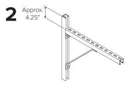
Mount the remaining 24" Slotted Tracks horizontally and protruding from the wall so that the slotted surface of the Slotted Track is 4.25" below the top edge of the vertical 24" Slotted Track. Use the Knee Braces, Angle Brackets, and the Spring-loaded Nuts and Hex Head Cap Screws to secure the horizontal Slotted Track in place.
