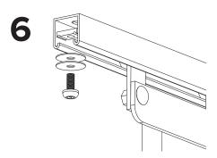
If no more Bike Files are going to be spliced together, insert a 3/8" Unistrut nut into the end of the channel and affix with 2 large washers and tamper-proof bolt. Finish by hammering in an End Cap.
