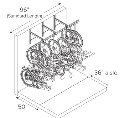
Bike Files may be lined up end to end to fill the available space. A 36" aisle should be left between the ends of bikes in racks facing one another.
