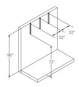
Mount 24" Slotted Tracks vertically to the wall with the appropriate anchors. Use a level for greatest accuracy. The bottom edge of the Slotted Track should be approximately 72" off the floor. The Slotted Tracks should be 32" apart from each other, and the end Slotted Tracks should be 18" from the eventual position of the end of the Trolley track.
