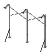
A) For single-sided units, attach Knee Braces to the first Upright and then every other Upright with  $3/8" \times 3"$  bolts, 3/8" washers, 3/8" lock washers, and 3/8" nuts. Anchor each Knee Brace by drilling a 3/8" hole and fastening with a wedge anchor.
