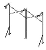
Fasten the Channel Supports to the uprights with 1/2" x 3" bolts, 1/2" washers, 1/2" lock washers, and 1/2" nuts.
