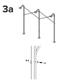
A) For single-sided units, fasten the Upright Braces to the Uprights with 3/8" x 3" bolts, 3/8" washers, 3/8" lock washers, and 3/8" nuts.
