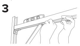
Make sure the horizontal Slotted Track is level. Adjust if necessary.
