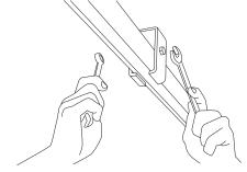
Secure the Channel Trolley Supports onto the 96" Slotted Track by tightening the Hex Head Cap Screws and Flange Nuts through the holes in the Channel Trolley Supports.
