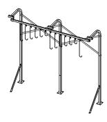
Insert the Track Rack or Bike File assembly into the Channel Supports and secure. See Track Rack or Bike File instructions for more detail.
