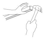
Insert a ½" Carriage Bolt into the last slot and fasten 3 Washers and a Tamperproof Nut. Finish by hammering in an End Cap.
