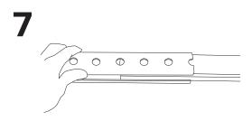
If splicing an additional length of track, slide the Splice Slotted Track over the last 6" of the 96" Slotted Track.
