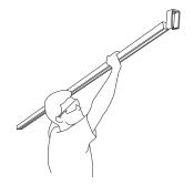
Slide 96" Slotted Track through the Channel Trolley Supports so that the centers of the brackets are 19" from the end of the Slotted Track.
