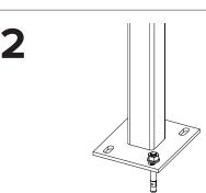
Anchor each Upright by drilling 3/8" holes and fastening with wedge anchors.
