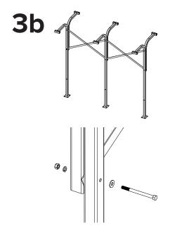
B) For double-sided units, fasten the Double-sided Uprights and Upright Braces to the Uprights with  $3/8" \times 3"$  bolts, 3/8" washers, 3/8" lock washers, and 3/8" nuts.
