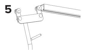
Insert the Trolleys into the open end of the 96" Slotted Track.
