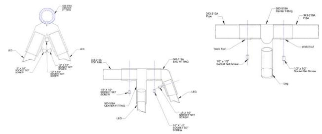
Note: Combination of a 583-518A center fitting and a 583-519A End Fitting is required for a complete Primary Tripod Swing End Fitting.
