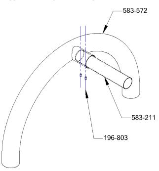
STEP #2: Remove swing hanger pendulums from the swing hanger assemblies. Using S-hooks, attach seats to chain and chain to swing hanger pendulums. Close the S-hooks to within .034" (1/32") using S-hook pliers.
