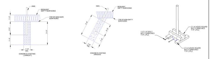
IF RESILIENT SURFACING IS TO BE LESS THAN 12", THEN ADDITIONAL PIPE SHOULD BE PUT IN CONCRETE TO MAINTAIN PROPER FINISH GRADE FOR EQUIPMENT.
