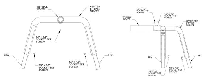
Note: Weld nuts on toprail do not line up with weld nut on fitting. Weld nuts shown on top for illustration purposes only, should be on side or bottom below horizontal so set screws point downwards. See center fitting detail.
