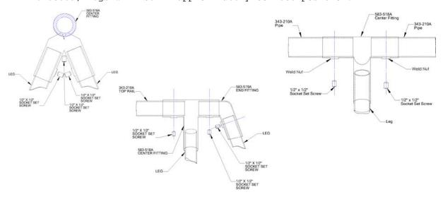
Note: Combination of a 583-518A center fitting and a 583-519A End Fitting is required for a complete Primary Tripod Swing End Fitting.
