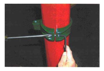
Decks attach to deck clamps using  $\frac{1}{2}$ " X 2  $\frac{1}{2}$ " Button Head bolts washer on top and bottom, with  $\frac{1}{2}$ " lock nuts. Connect the deck bolt firmly.
