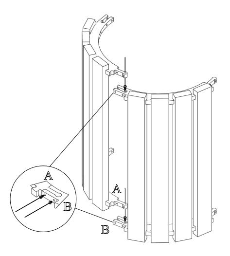
Step 1: Take Panel A and place it in the vertical position, align panel B with panel A in the vertical position making sure the rail aligns with the top and the bottom. Slide the rails in a downward motion until they are even. Make sure the holes in the rails are aligned.
