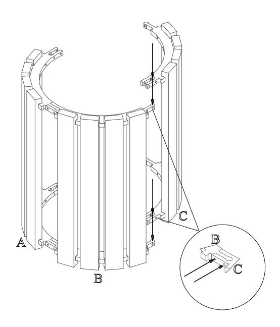
Step 2: Take Panel C place it in the vertical position, aligning it with Panels A and B. slide the rail of panel C in a downward motion and align the holes in the rail.
