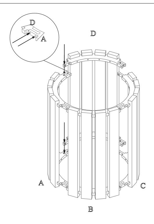
Step 3: Take Panel D place it in the vertical position, aligning it with Panels A, B and C. Slide the rail of panel D in a downward motion and align the holes in the rail.
