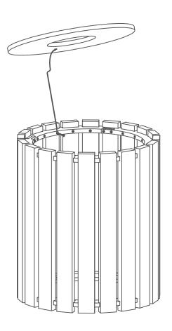
Step 5: If you would like to take advantage of the supplied Lid Lanyard, just remove the desired screw from the top rail and re-secure it with the lanyard attached. Just remove the screw in the lid if you would like to forgo the use of the Lid Lanyard.
