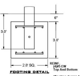
\*Footing design based on 1500 PSF soil bearing pressure.
