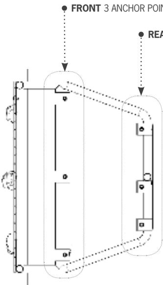
6 REQUIRED ANCHORING BRACKET POSITIONS FIGURE G
