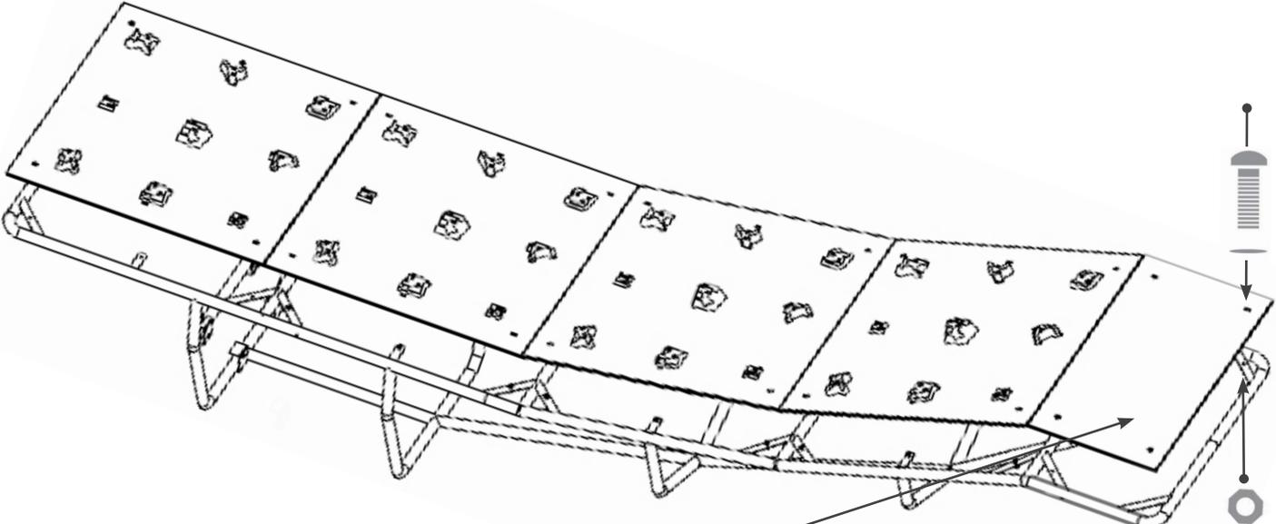
**Affix the 2' x 4' safety panel to the top of the climbing frame using:**
