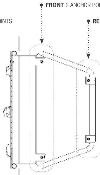
4 REQUIRED ANCHORING BRACKET POSITIONS FIGURE G
