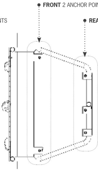
5 REQUIRED ANCHORING BRACKET POSITIONS FIGURE G
