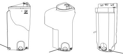
**Step 2:** Using a drill with a 1-3/4" hole saw, drill a hole in the location where the new drain plug is to be located. Clean any burrs or shavings off of the edge of the hole.
