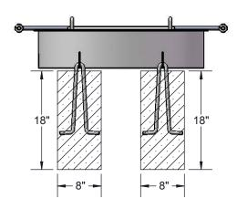
Attach the ground staples to the Fire Ring before inserting then into the concrete footings.
