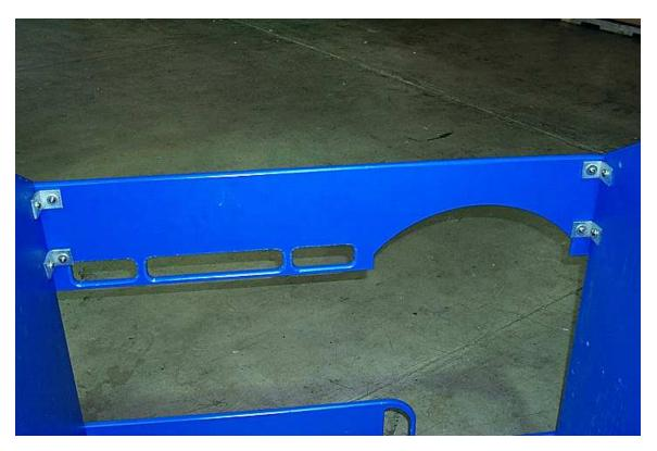
6. Install 3 corner brackets in the lower 3 holes of the back panel (A) and 1 bracket on the side counter panel (B) near the back towards the back panel (A). Now attach the large seat (F) on these 4 brackets with 5/16" x <sup>3</sup>/<sub>4</sub>" bolt, 5/16" x 1" nut, 5/16" washer, and 3/8" washer and tighten all hardware along this side, making sure the corners are flush with one another.
