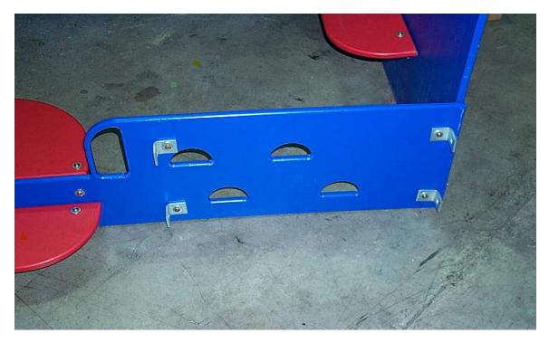
13. Now install the ladder support triangles to the previously installed corner brackets and then install 4 corner brackets to the remaining 4 holes in the triangles with the brackets facing to the inside.
