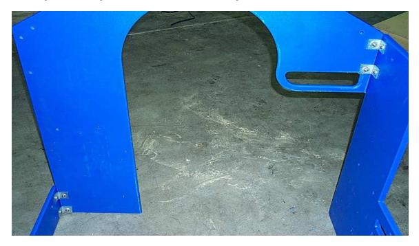
5. Install 2 corner brackets to the upper 2 holes on the side of the front entry panel. Attach the upper side panel (E) above the lower side panel (C) with the 4 previously installed corner brackets.
