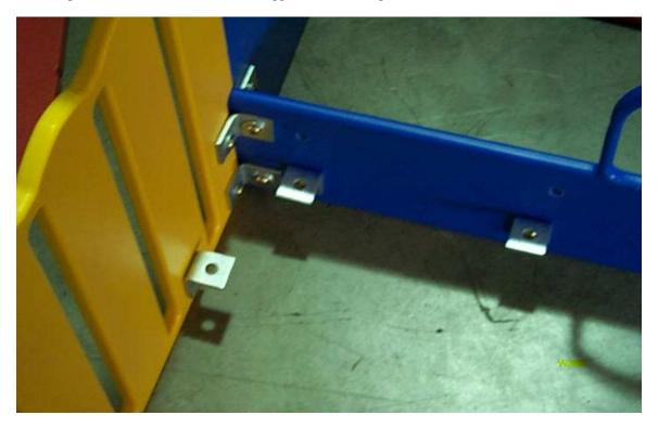
8. Next install 2 corner brackets to the upper 2 holes in the lower side panel (C) and 1 corner bracket in the lower hole of the front entry panel (D). These brackets will support the large step (H). Once these brackets are install place the small step (I) on the corner brackets from step 7 and install the large step on the remaining 3 corner brackets. Tighten all hardware on this corner.
