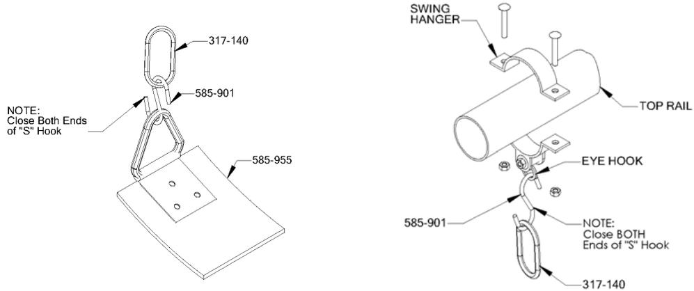
STEP #3: Assemble top portion of swing hangers on top rail following spacing on page 1 diagram.
