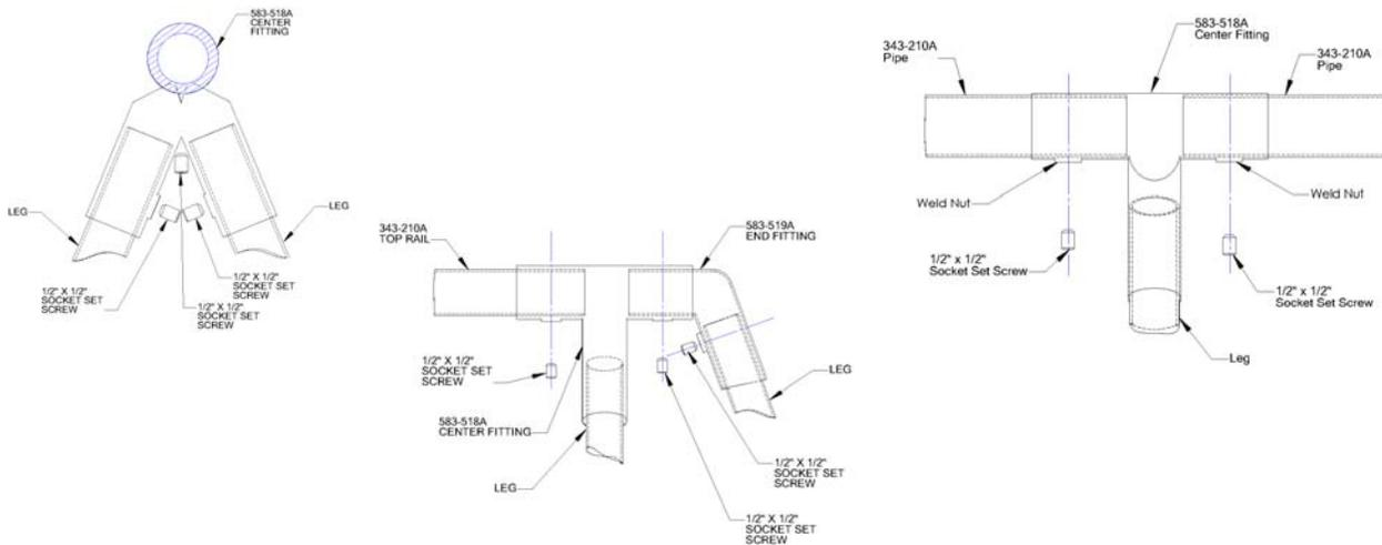
Note: Combination of a 583-518A center fitting and a 583-519A End Fitting is required for a complete Primary Tripod Swing End Fitting.
