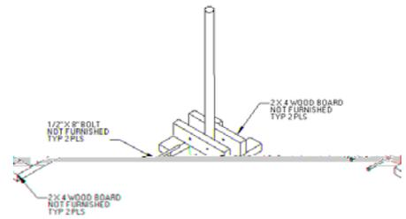
**IF RESILIENT SURFACING IS TO BE LESS THAN 12", THEN ADDITIONAL PIPE SHOULD BE PUT IN CONCRETE TO MAINTAIN PROPER FINISH GRADE FOR EQUIPMENT.**
