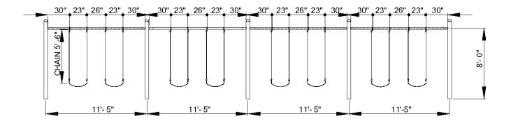
To insure proper swing height, install to an 8' height, measuring from the top of the resilient surfacing to the bottom of the top rail.
