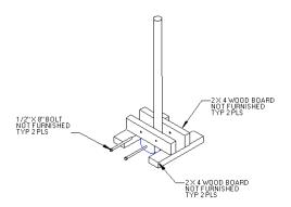
IF RESILIENT SURFACING IS TO BE LESS THAN 12", THEN ADDITIONAL PIPE SHOULD BE PUT IN CONCRETE TO MAINTAIN PROPER FINISH GRADE FOR EQUIPMENT.
