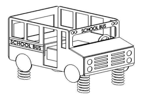
**<u>NOTE</u>**: Picture differs slightly from the actual product, the center seats have been replaced with a divider. This instruction set is for a stationary school bus, the springs are replaced with 4 pipes to be set in concrete.
