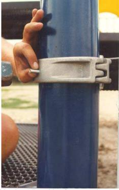
into the posts with a  $\frac{1}{4}$ " metal drill bit. Install the  $\frac{3}{4}$ " roll pins so that they are "flush" with the posts.
