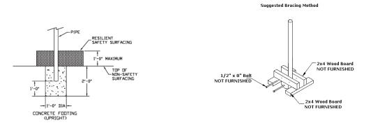
• If resilient surfacing is to be less than 12", then additional pipe should be put in concrete to maintain proper finish grade for equipment.
